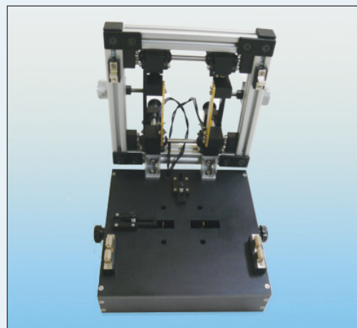
FIGURE 8: FRONT VIEW OF THE FIXTURE WITH TOP CONTACTS RAISED
