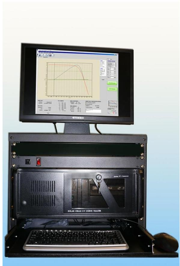
Figure 3: Typical I-V System Console
