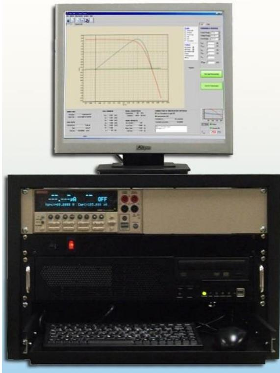
Figure 2: Typical I-V System Console
