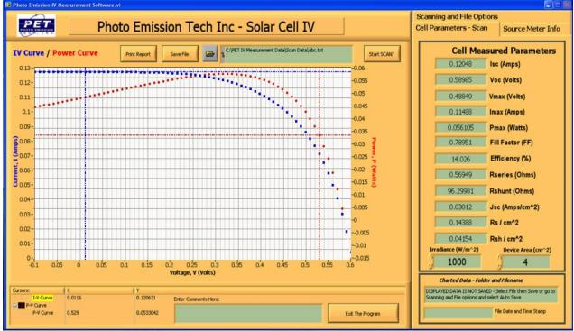
Figure 4: Cell Parameter Scan Screen
