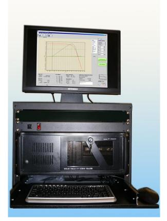
Figure 3: Typical I-V System Console - 15A/20A Current
